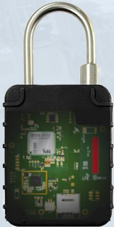
In-built iSIM card and Telit 310G module (modem)
